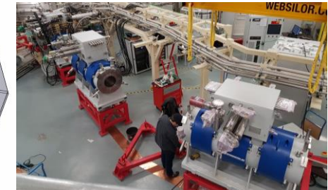
Superconducting Multipole Triplets and Power-Supply Systems (x7)
